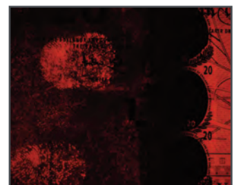
DFO treated fingerprints on banknote viewed under orange illumination
