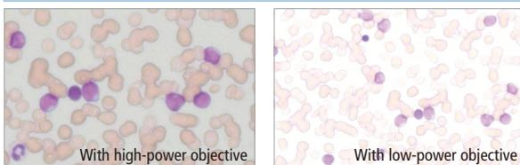
Since brightness varies depending on the objective, switching magnifications can induce eye strain.
