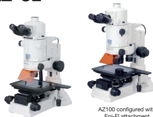
AZ100M configured with Epi-Fl attachment
